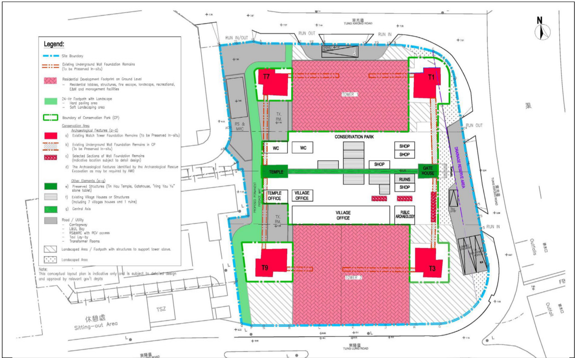
Figure 46. Tentative Conceptual Layout Plan from Ground Level to 21.9mPD showing boundary of Conservation Park (subject to change in detail design stage)
